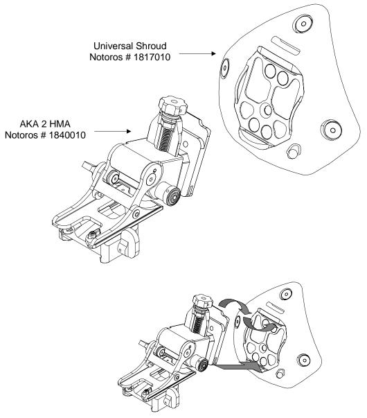
**Helmet Mount Attachment:** Push the top of the helmet mount into the top of the bracket shroud. Push the bottom of the mount down into the bracket shroud until it snaps locked.
